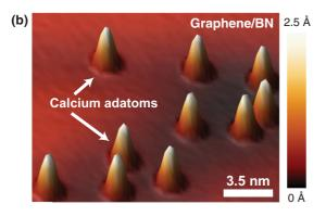
FIG. 1. (a) Schematic of the experimental setup. Calcium atoms are deposited onto a graphene/BN/SiO<sub>2</sub>/Si device. A voltage  $V_{\rm g}$  is applied to Si to tune the charge-carrier density in graphene, and a voltage  $-V_{\rm s}$  is applied to the STM tip. (b) STM topographic image of Ca atoms adsorbed onto a graphene/BN surface.
